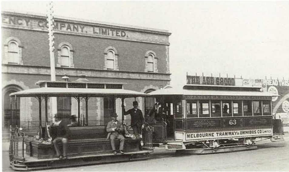
Cable tram of the Melbourne Tramway and Omnibus Company. The gripman and the more adventurous passengers rode the open 'dummy' or grip car at the front, while the rest rode with the conductor in the saloon or trailer car. Cable trams were powered by a continuously moving underground cable driven by a stationary steam engine. The tram was attached to the cable by means of the grip through a slit in the roadway.
